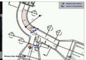
Wireless tags will send an alert if a worker stops moving for a set period of time. They can also alert workers if they are too close to the moving plant, or sound a warning if unauthorised personnel enter hazardous zones, such as a storage area for explosives.
