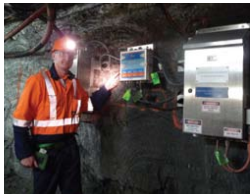
Wireless tags will send an alert if a worker stops moving for a set period of time. They can also alert workers if they are too close to the moving plant, or sound a warning if unauthorised personnel enter hazardous zones, such as a storage area for explosives.
